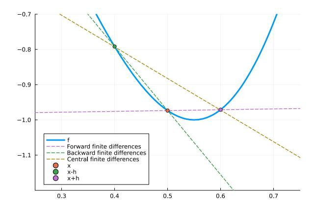
Let us consider the convergence of these three variants for computing the derivative of  $f(x)=e^{\sin(x)}$  at x=0. First we construct the range of h values:
