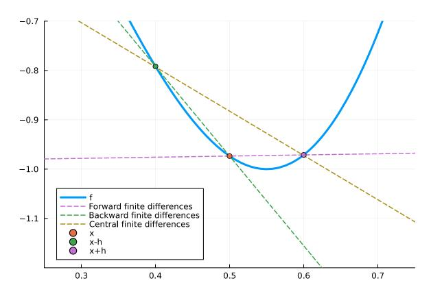
In this image the value of the finite-difference derivative was the slope of the plotted lines. Most notably these lines are interpolating lines between two of the points (x-h, f(x-h)), (x, f(x)) or (x+h, f(x+h)).
