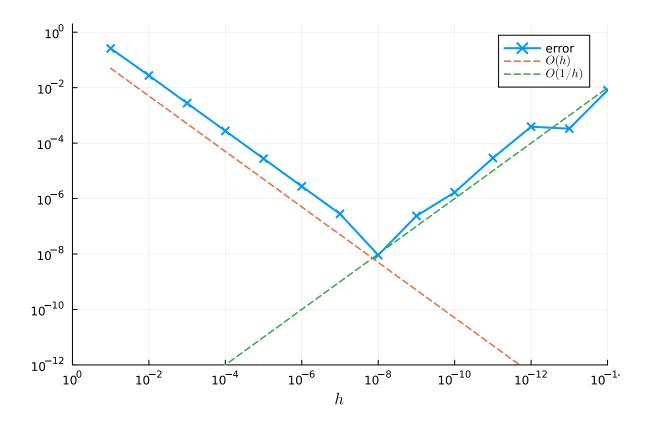
**Optimal** h for higher-order formulas: Note that in (6) the h dependence of the first error term (finite difference truncation error) depends on the order of the finite difference formula.
