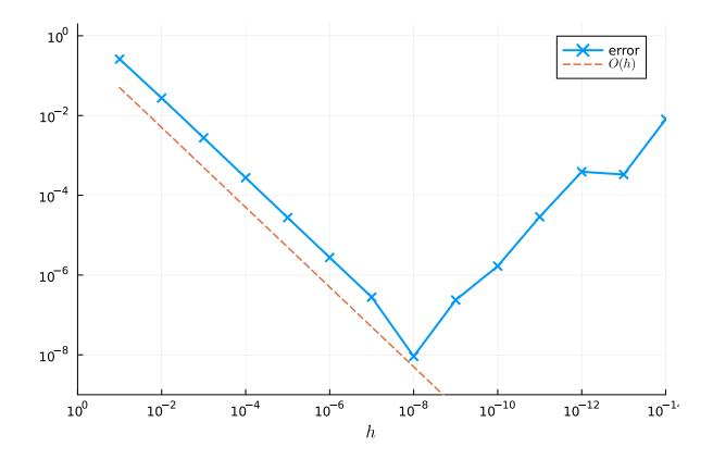
We notice that the derivative formula gives a good approximation to the exact derivative  $f'(0) = e \cos(e)$  for  $h = 10^{-8}$ . However, if the node distance h is further descreased the approximation deteriorates. This is a result of the round-off error in the finite-precision floating-point arithmetic of the computer as we will discuss now in more detail.
