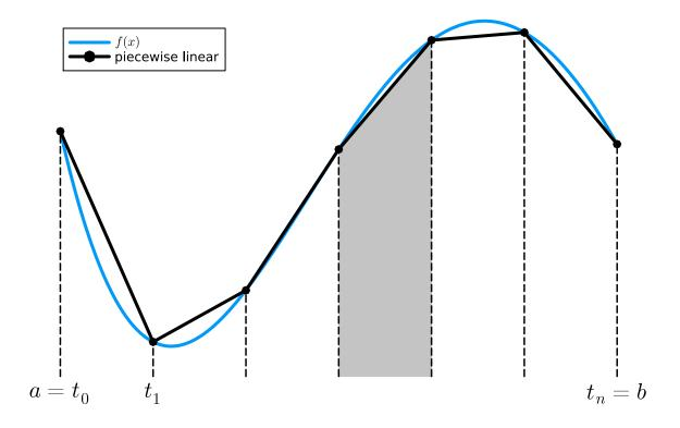
To approximate integral  $I=\int_a^b f(x)dx$ , that is the area under the blue curve, we evaluate the function f at n+1 equispaced nodes leading to data points  $(t_i,f(t_i))$ . From these we construct a piecewise linear polynomial interpolation  $p_{1,h}$  (black line). Integrating  $p_{1,h}$  on  $[t_0,t_n]$  then yields an approximation to I:
